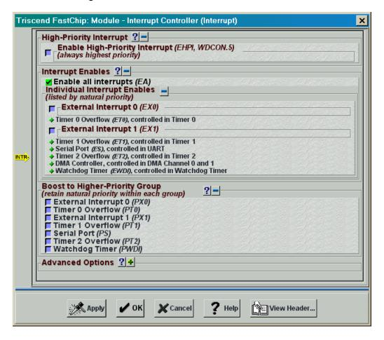
To enable the specific interrupt from the UART, click on the UART button in the Dedicated Resources area and then click on the Enable UART Interrupt checkbox in the **8032 UART** window. In addition to this, click on the Enable Receiver checkbox. This will move the enabling of the UART to the initialization subroutine so you don't have to do it explicitly at the beginning of the main() routine (see line 11 of Listing 3). Then click on OK to close the window.
