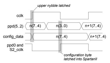
Once all the configuration data enters the SpartanII, it will raise its DONE pin. This will raise the chip-select and write-strobe of the SpartanII (lines 49–50) and disable further writing of configuration data. It will also make the CPLD release control of the SpartanII configuration data input pins (lines 54 and 55).
