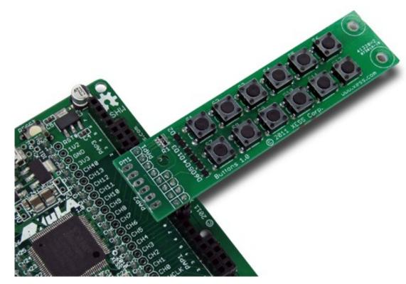
Then insert the module into one of the eight-bit Wing sockets on the StickIt! board.
