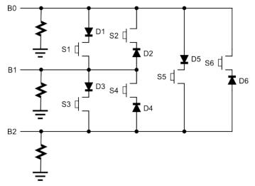
Driving signal B0 and sensing the level on B1 will detect whether button S1 is open or closed. If closed, then B1 is driven high by B0; if open, then B1 is pulled low by the attached pulldown resistor. In either case, the state of button S2 will not have any effect because diode D2 blocks B0 from driving B1.
