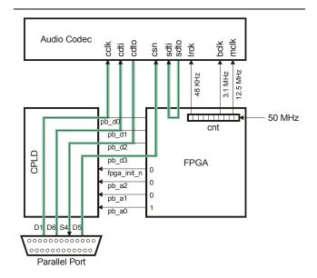
Figure 1: Codec parallel port interface schematic.
