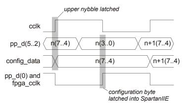
Once all the configuration data enters the SpartanIIE, it will raise its DONE pin. This activates the circuitry described on lines 59–83 that allows the SpartanIIE to communicate with the PC parallel port through the CPLD. The chip-select and write-strobe of the SpartanIIE are used to receive a clock and reset signal from the PC to the FPGA (lines 60 and 61, respectively). These signals control state machines that are loaded into the SpartanIIE.
