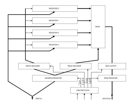
The FSM that controls the designed protocol is depicted in the figure. When READb or WRITEb is lowered the machine acts to read or write and waits for the rising edge. If the READb and WRITEb signals are lowed the machine waits for an address.
