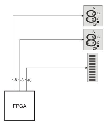
The table below lists the connections from the FPGA to the LEDs. The LEDs are attached through the Peripheral Bus so the other components on the bus must be tristated if a stable display is desired.
