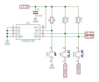
During normal operation, the EEPROM contents are read by the Raspberry Pi so that it can see what GPIO pins are used by the XuLA Board inserted in the StickIt! Board. In order to program the EEPROM with that information, you must place a shunt on the WP jumper to disable the write-protect function. The Raspberry Pi can then load the EEPROM through the ID\_SC and ID\_SD pins of the GPIO header. (Read more about this process on page 21.)
