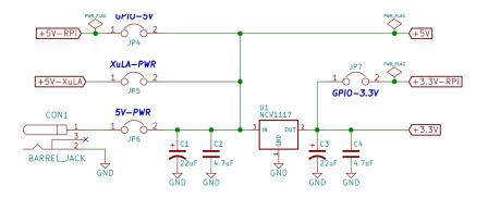
Be aware that placing shunts on both the XULA-PWR and 5V-PWR jumpers will connect the external power adapter to the XuLA Board power supply. **This will cause damage** unless 1) the USB cable is removed from the XuLA Board, or 2) the 5V jumper on the XuLA Board is open. (Note that in its factory-original configuration, the 5V jumper on the XuLA Board is shorted by a wiring trace on the bottom of the PCB which must be cut to disconnect the 5V supply from the USB port.)
