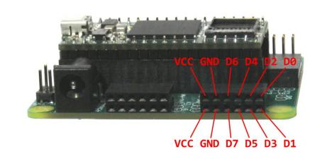
The physical arrangement of the PMOD I/O signals is shown below.
