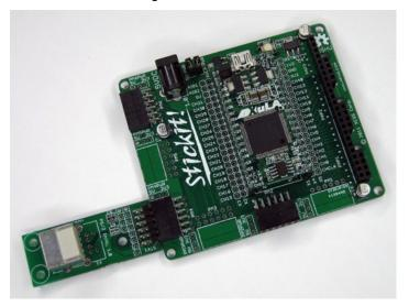
All of these sockets (PM1 - PM6) accept either four-bit or eight-bit PMOD modules.
